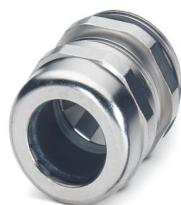
Cable gland, material for screw connection: Brass, nickel-plated, application: EMC, external cable diameter 14 mm ... 21 mm, shielding: yes, connecting thread: M32 x 1.5, color: silver, with O-ring
