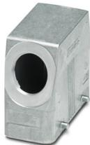
Sleeve housing B16, for double locking latch, material: Die-cast aluminum, salt water resistant, cable outlets: 1, lateral, 1x M32, height: 76 mm, cable gland: none, Standard
