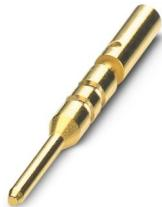
Crimp contact, Pin, turned, contact diameter: 0.8 mm, crimp range: 0.34 mm<sup>2</sup> ... 0.5 mm<sup>2</sup>,
