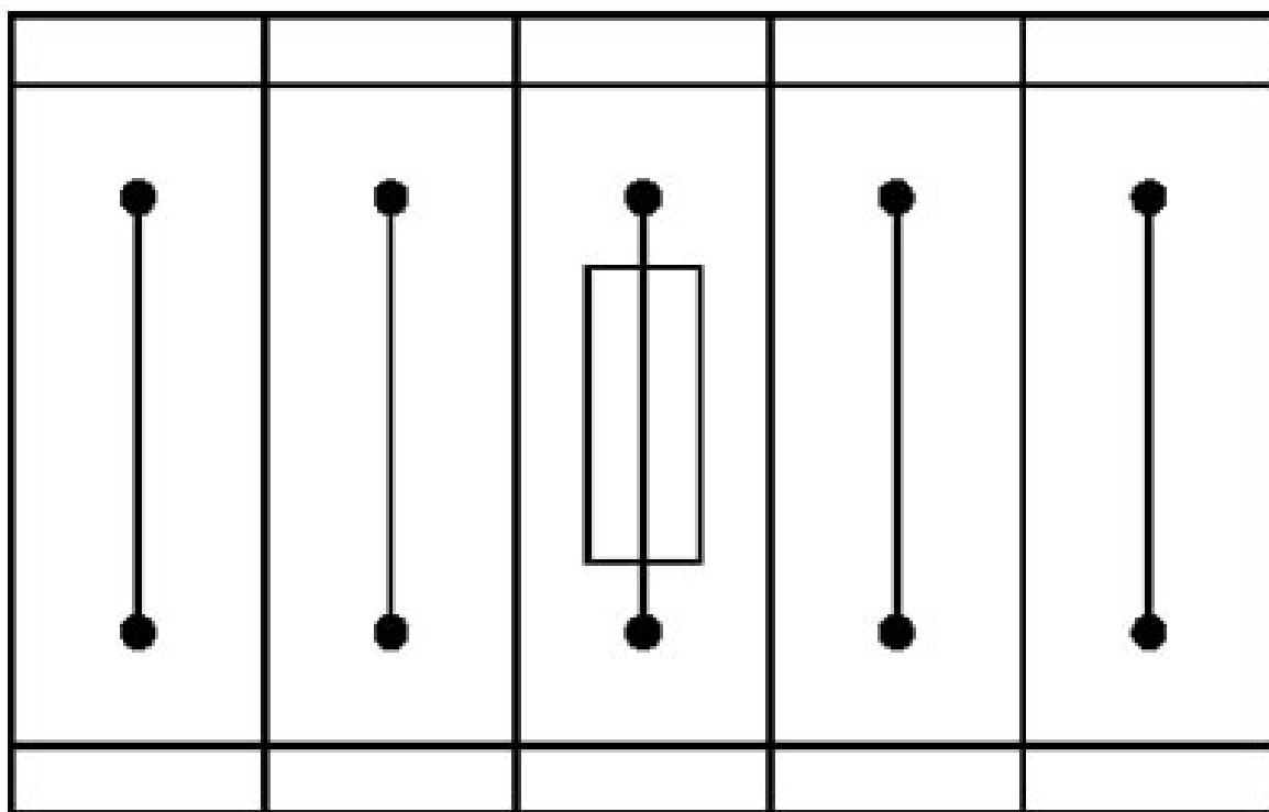
Fuse terminal block in single arrangement,
