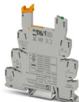
6.2 mm PLC basic terminal block with screw connection, without relay or solid-state relay, for mounting on DIN rail NS 35/7,5, 1 changeover contact, input voltage 230 V AC/DC
