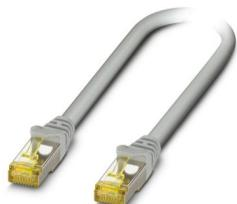
Patch cable, degree of protection: IP20, cable length: 2 m, number of positions: 8, 10 Gbps, CAT6<sub>A</sub>, connection method: Pierce connection, connection cross section: AWG 26- 26, cable outlet: straight, Ethernet
