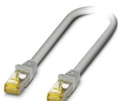
Patch cable, degree of protection: IP20, cable length: 3 m, number of positions: 8, 10 Gbps, CAT6<sub>A</sub>, connection method: Pierce connection, connection cross section: AWG 26- 26, cable outlet: straight, Ethernet
