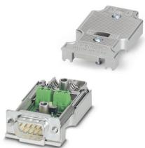
D-SUB connector, 9-pos., male connector, axial version with two cable entries, bus system: PROFIBUS DP up to 12 Mbps, termination resistor can be switched on via slide switch, pin assignment: 3, 5, 6, 8; screw connection terminal blocks
