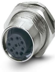
Device connector rear mounting, 8-position, Socket, M12, coding: A, Rear mounting, M16 x 1.5, Wave soldering, Alternative product in accordance with RoHS II without Exemption 6c (Pb < 0.1 %) item no.: 1239740
