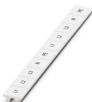
Marker for terminal blocks, Strip, white, labeled, can be labeled with: CMS-P1-PLOTTER, horizontal: L1, L2, L3, N, PE, L1, L2, L3, N, PE, mounting type: snapped, for terminal block width: 10.2 mm, lettering field size: 10,15 x 10,5 mm, Number of individual labels: 10
