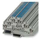
Feed-through terminal block, nom. voltage: 500 V, nominal current: 24 A, connection method: Spring-cage connection, 1st, 2nd and 3rd level, Rated cross section: 2.5 mm<sup>2</sup>, cross section: 0. 08 mm<sup>2</sup> - 4 mm<sup>2</sup>, mounting type: NS 35/7,5, NS 35/15, color: gray
