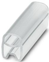
Conductor marker carrier, transparent, unlabeled, mounting type: slide-on, cable diameter range: 1.5 ... 2.5 mm, lettering field size: 15 x 4 mm
