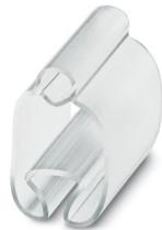
Conductor marker carrier, transparent, unlabeled, mounting type: slide-on, cable diameter range: 10 ... 14 mm, lettering field size: 15 x 4 mm
