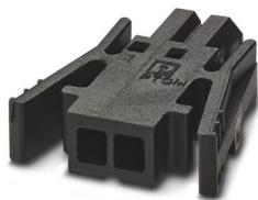
PCB connector, nominal cross section: 0.75 mm<sup>2</sup>, color: black, nominal current: 6 A, rated voltage (III/2): 160 V, contact surface: Tin, contact connection type: Socket, number of rows: 1, number of positions: 2, product range: PTCM 0,5/..-PL, pitch: 2.5 mm, connection method: Crimp connection, conductor/PCB connection direction: 0 °, plug-in system: COMBICON PTSM, locking: Snap-in locking, mounting: Self-locking flange, type of packaging: packed in cardboard
