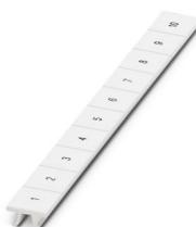
Zack marker strip, Strip, white, labeled, can be labeled with: CMS-P1-PLOTTER, printed horizontally: consecutive numbers 1 ... 10, 11 ... 20, etc. up to 91 ... 100, mounting type: snapped, for terminal block width: 10.2 mm, lettering field size: 10,15 x 10,5 mm, Number of individual labels: 10
