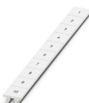
Zack marker strip, Strip, white, labeled, can be labeled with: CMS-P1-PLOTTER, Printed vertically: consecutive numbers 1 ... 10, 11 ... 20, etc. up to 91 ... 100, mounting type: snapped, for terminal block width: 10.2 mm, lettering field size: 10,15 x 10,5 mm, Number of individual labels: 10
