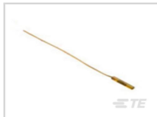
NTC Sensor Type: **Epoxy Coated NTC Thermistor**Lead Wire Length: **152 mm [ 5.984 in ]**Resistance (at 25°C): **2 kΩ**β-Value(25/85): **3499 K**Tolerance β-Value: **±.5 %**[All Thermistor Probe - Micro BetaCHIP \(MCD\) \(3\)](#)
