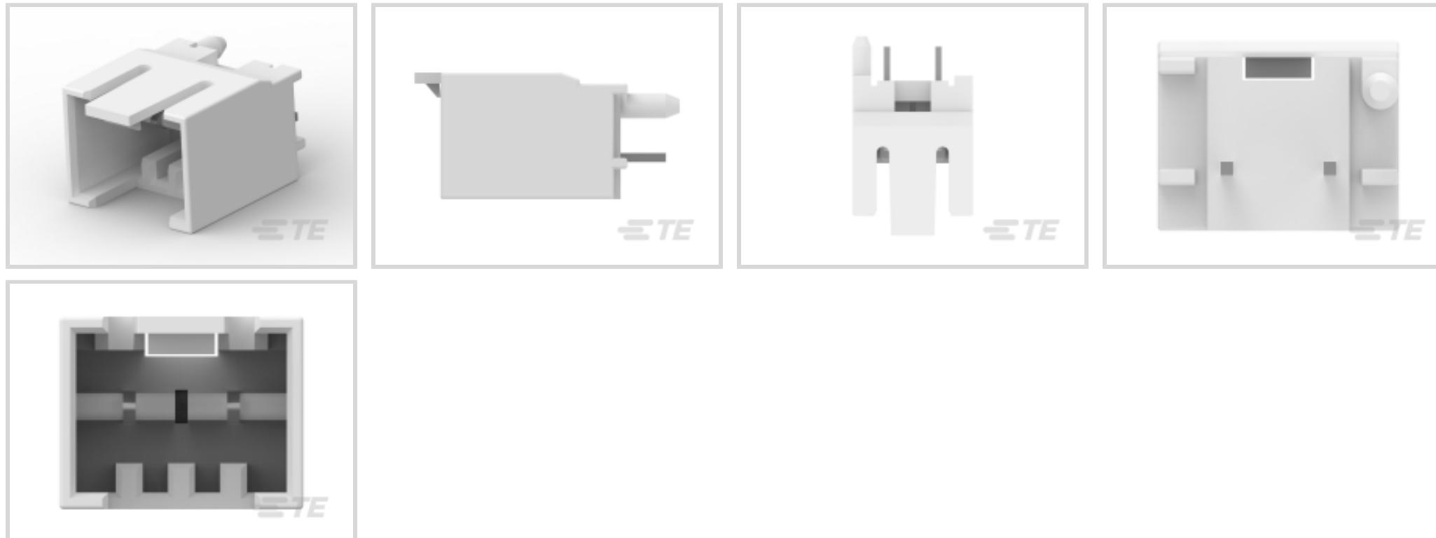
Connector System: **Wire-to-Board**Number of Positions: **3**Number of Rows: **1**Centerline (Pitch): **5 mm [.197 in]**PCB Mount Orientation: **Vertical**
