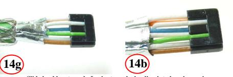
Slide load bar to end of pairs to make loading into housing easier
