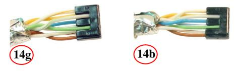
Slide load bar to end of pairs to make loading into housing easier
