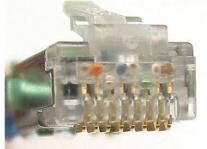
Verify wires are visible through end of plug
