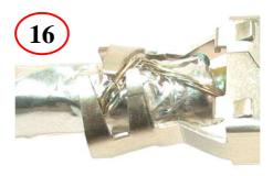
Close shield fingers by hand Keep drain wire entirely under fingers
