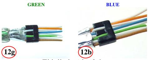
Slide load bar down to base of pairs
