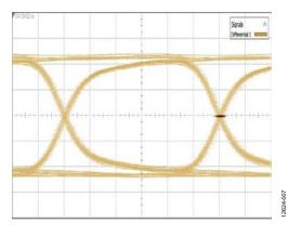
Figure 7. Output Eye Diagram at CPRI  $\times$  12 = 6.144 Gbps, Time = 27.13 ps/div, Amplitude = 118 mV/div
