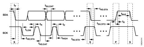
Figure 14. I<sup>2</sup>C Interface Timing Diagram
