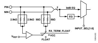
Figure 22. Input Stage Block Diagram
