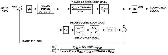
Figure 15. CDR Jitter Block Diagram
