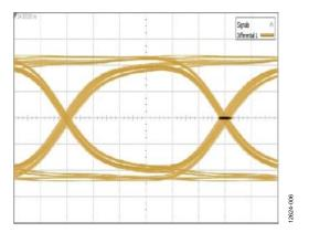
Figure 6. Output Eye Diagram at  $CPRI \times 16 = 9.8304$  Gbps, Time = 16.95 ps/div, Amplitude = 116 mV/div
