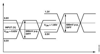
Figure 28. Minimum Allowed DC-Coupled Input Levels
