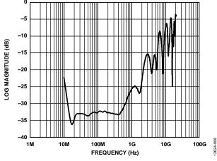
Figure 8. Typical S11 Spectrum Performance
