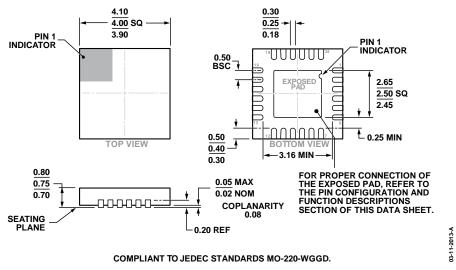
Figure 30. 24-Lead Lead Frame Chip Scale Package [LFCSP] 4 mm × 4 mm Body and 0.75 mm Package Height (CP-24-7) Dimensions shown in millimeters
