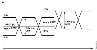
Figure 29. Maximum Allowed DC-Coupled Input Levels
