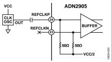
Figure 20. AC-Coupled, Single-Ended REFCLKx Configuration
