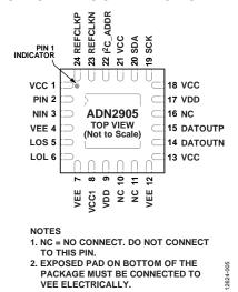
Figure 5. Pin Configuration
