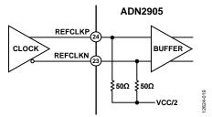
Figure 19. DC-Coupled, Differential REFCLKx Configuration
