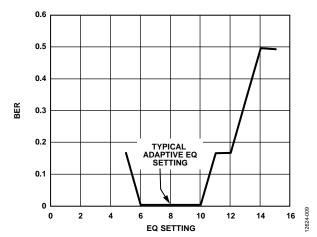
Figure 9. BER in Equalizer Mode vs. EQ Compensation at CPRI × 16 = 9.8304 Gbps (with a Signal of 400 mV p-p Differential, on 15 inch FR4 Traces, with Variant EQ Compensation, Including Adaptive EQ)
