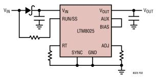
Figure 2. The Input Diode Prevents a Shorted Input from Discharging a Backup Battery Tied to the Output. It Also Protects the Circuit from a Reversed Input. The LTM8025 Runs Only When the Input is Present.
