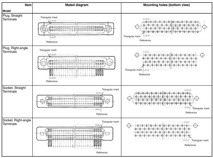
Contact numbers are not printed on the connectors. Use the triangular mark (♥) as a guide when designing and mounting to boards. • On the mating side, the row of terminals on the triangular mark side are called row a, and the row on the other side is called row b. The numbers are in the order shown. • The triangular marks on the plug and socket must be aligned when mated. The contact numbers on both sides must match.
