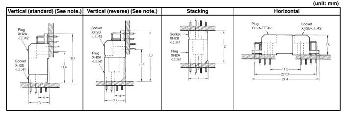
Note: The function of the standard and reverse models is the same as that of the standard XC5 DIN Connector.
