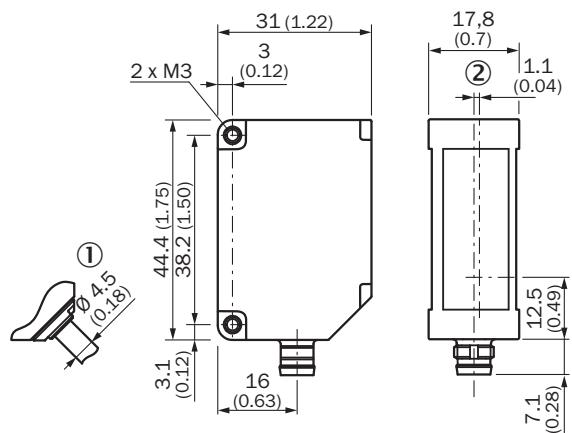
① Variant with 30 cm cable with M12, 5-pin connector
