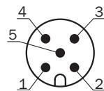
Connector M12, 5-pin, A-coded
