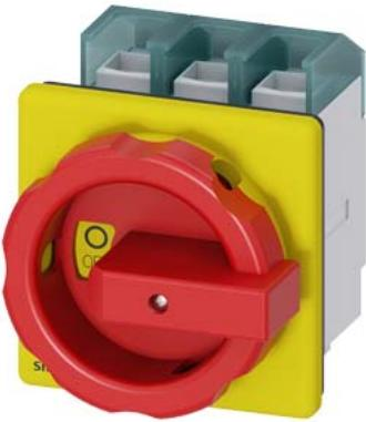
SENTRON, Switch disconnector 3LD, emergency switching-off switch, 3-pole, I<sub>u</sub>: 125 A, operating power / at AC-23 A 400 V: 45 kW, front-mounted, rotary operating mechanism, Red / yellow, 4-hole mounting of the handle
