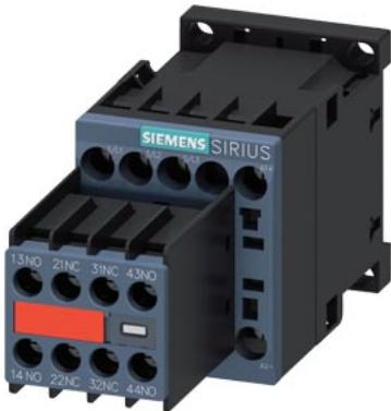
Power contactor, AC-3 12 A, 5.5 kW / 400 V 2 NO + 2 NC, 24 V DC 3-pole, Size S00 Screw terminal Captive auxiliary switch
