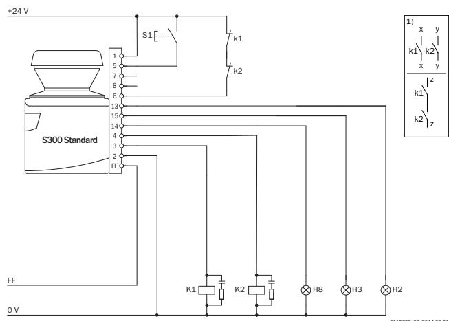
S300 Standard in conjunction with relays/contactors
