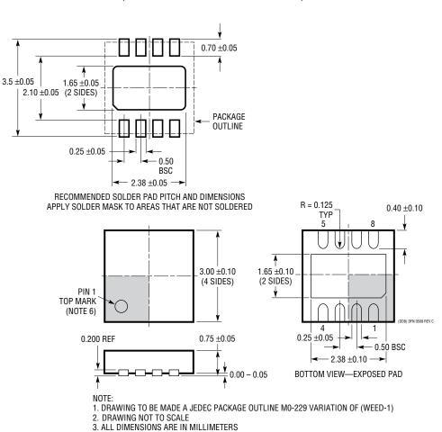
**DD Package** 8-Lead Plastic DFN ( $3mm \times 3mm$ ) (Reference LTC DWG # 05-08-1698 Rev C)
