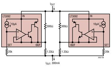
Figure 8. Connect Two LT3092s for Higher Current
