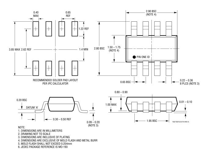
TS8 Package 8-Lead Plastic TS0T-23 (Reference LTC DWG # 05-08-1637 Rev A)
