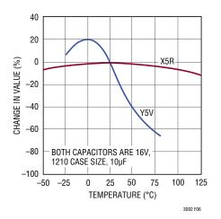
Figure 6. Ceramic Capacitor Temperature Characteristics
