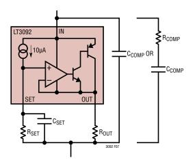
Figure 7. Adding  $C_{SET}$  Lowers Current Noise
