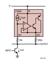
Pulsed Current Source, Load to Ground
