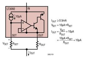
Figure 1. Using the LT3092 as a Current Source
