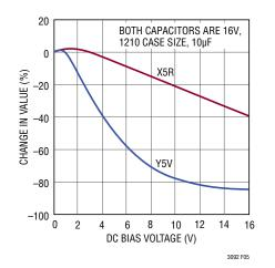
Figure 5. Ceramic Capacitor DC Bias Characteristics
