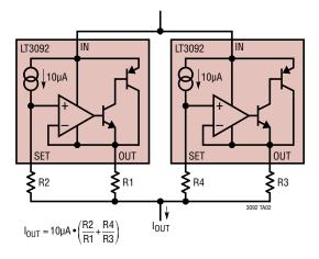
Paralleling LT3092s with Ballast Resistor
