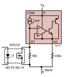
Pulsed Current Source, Load to  $V_{\rm IN}$
