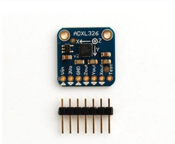
The ADXL326 can measure at least +/- 16G(!) in the X, Y and Z axis. It is ideal for measuring more dynamic accelerations from high-performance land and air vehicles as well as for shock and impact measurements.
