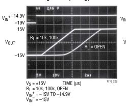
Below V<sub>S</sub><sup>-</sup> Fault (Falling)
