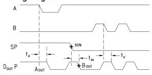
td = propagation delay, A or B to Dout tds = propagation delay, Select to Dout
