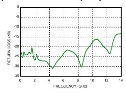
**Output Return Loss vs. Frequency**
