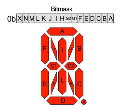
The bitmask is a 16-bit number that can be passed in as a single Hexidecimal, Decimal, or binary number. It can also be passed in as a list or tuple containing 2 separate 8-bit numbers. Here are some of the ways to set the digits. All of these different methods create a box with an X in the center:
