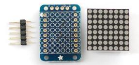
When you buy a pack from Adafruit, it comes with the fully tested and assembled backpack as well as a 8x8 matrix in one of the colors we provide (say, red, yellow or green). You'll need to solder the matrix onto the backpack but its an easy task.
