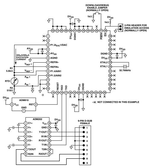
Figure 53. Typical System Configuration
