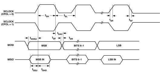
Figure 9. SPI Master Mode Timing (CPHA = 0)
