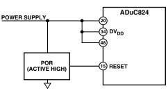
Figure 48. External Active High POR Circuit
