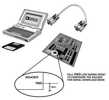
Figure 28. Flash/EE Memory Serial Download Mode Programming
