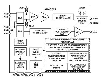
low-level signals). The ADCs with on-chip digital filtering are intended for the measurement of wide dynamic range, low-frequency signals, such as those in weigh scale, strain-gauge, pressure transducer, or temperature measurement applications. The ADC output data rates are programmable and the ADC output resolution will vary with the programmed gain and output rate.
