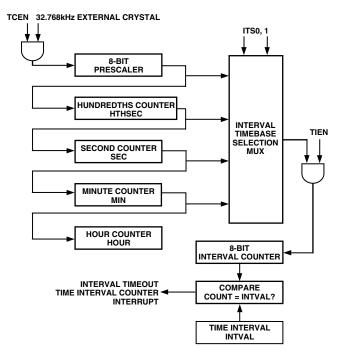
Figure 32. TIC, Simplified Block Diagram
