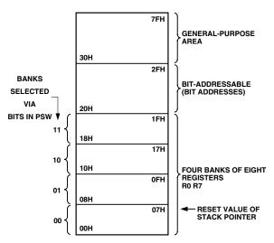
Figure 15. Lower 128 Bytes of Internal Data Memory
