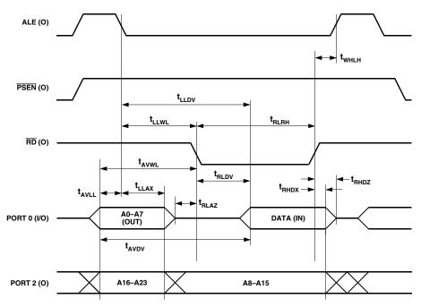
Figure 4. External Data Memory Read Cycle
