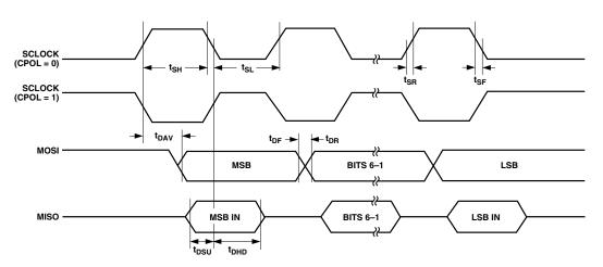
Figure 8. SPI Master Mode Timing (CPHA = 1)
