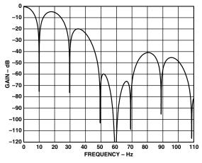
Figure 22. Filter Response, SF = 69 dec
