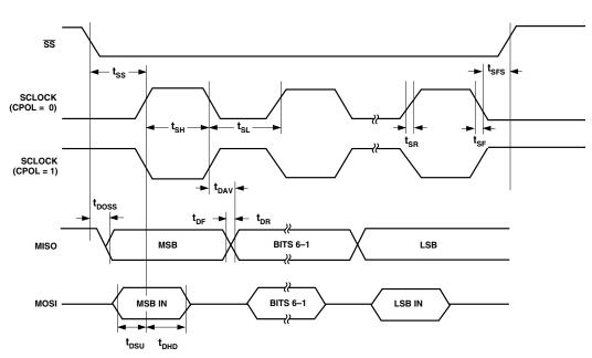
Figure 11. SPI Slave Mode Timing (CPHA = 0)
