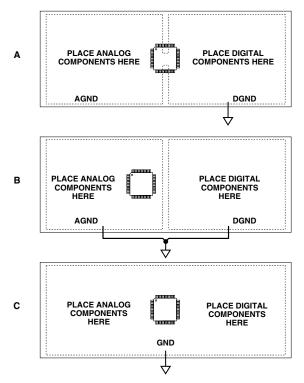
Figure 52. System Grounding Schemes
