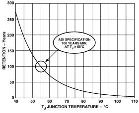
Figure 27. Flash/EE Memory Data Retention
