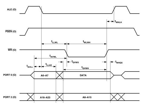
Figure 5. External Data Memory Write Cycle
