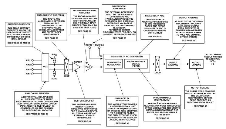
Figure 18. Primary ADC Block Diagram
