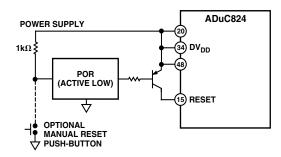
Figure 49. External Active Low POR Circuit
