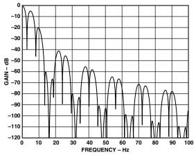
Figure 23. Filter Response, SF = 255 dec
