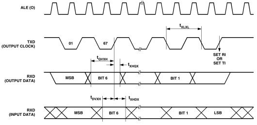
Figure 6. UART Timing in Shift Register Mode
