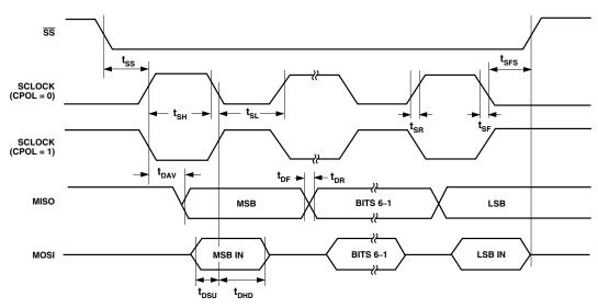
Figure 10. SPI Slave Mode Timing (CPHA = 1)
