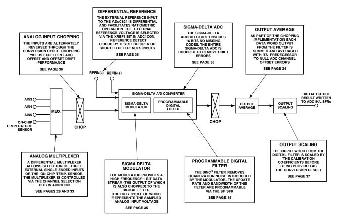
Figure 19. Auxiliary ADC Block Diagram
