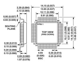
CONTROLLING DIMENSIONS ARE IN MILLIMETERS; INCH DIMENSIONS (IN PARENTHESES) ARE ROUNDED-OFF MILLIMETER EQUIVALENTS FOR REFERENCE ONLY AND ARE NOT APPROPRIATE FOR USE IN DESIGN
