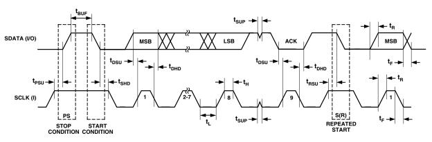
Figure 7. I<sup>2</sup>C-Compatible Interface Timing
