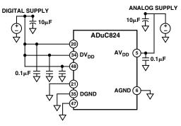
Figure 50. External Dual Supply Connections
