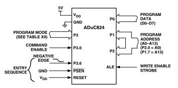
Figure 29. Flash/EE Memory Parallel Programming
