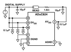
Figure 51. External Single Supply Connections
