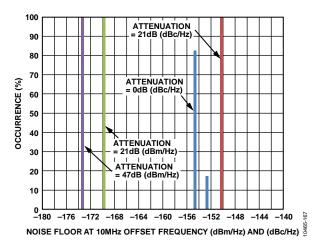
Figure 21. Noise Floor at 10 MHz Offset Frequency Distribution at Worst-Case Conditions and Different Attenuation Settings
