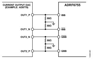
Figure 61. Establishing DC Bias Level on Baseband Inputs
