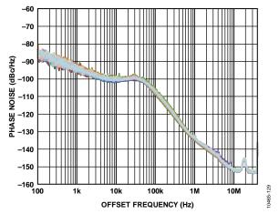
Figure 29. Phase Noise Performance Distribution at Worst-Case Conditions
