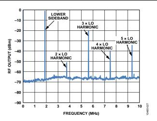
Figure 26. RF Output Spectral Plot over a Wide Span
