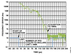
Figure 35. PLL Frequency Settling Time at Worst-Case LO Frequency with Lock Detect Shown
