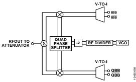
Figure 60. Block Diagram of the Quadrature Modulator
