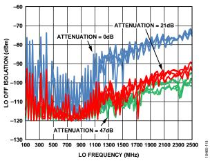
Figure 17. LO Off Isolation vs. LO Frequency, Attenuation, Supply, and Temperature
