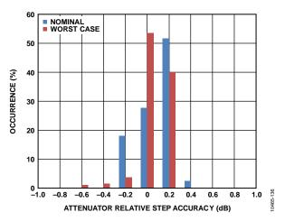
Figure 38. Attenuator Relative Step Accuracy Distribution at Nominal and Worst-Case Conditions, LO > 300 MHz, All Attenuation Steps
