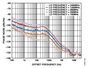
Figure 27. Phase Noise Performance vs. LO Frequency, Nominal Conditions
