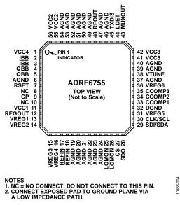
Figure 4. Pin Configuration
