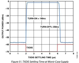
re 51. TXDIS Settling Time at Worst-Case Suj and Temperature
