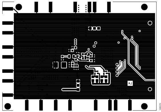
Figure 75. Evaluation Board, Bottom Side—Layer 4
