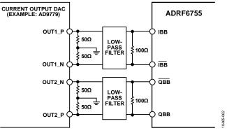
Figure 62. Typical Baseband Input Configuration
