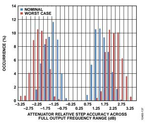
Figure 39. Attenuator Relative Step Accuracy Across Full Output Frequency Range Distribution at Nominal and Worst-Case Conditions, LO > 300 MHz, All Attenuation Steps
