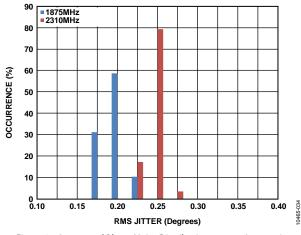
Figure 31. Integrated Phase Noise Distribution over an Integration Bandwidth of 1 kHz to 8 MHz at 1875 MHz and 2310 MHz
