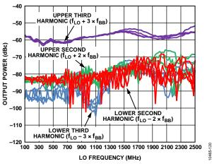
Figure 19. Second-Order and Third-Order Harmonic Distortion vs. LO Frequency, Supply, and Temperature
