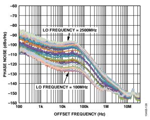
Figure 28. Phase Noise Performance vs. LO Frequency, Supply, and Temperature
