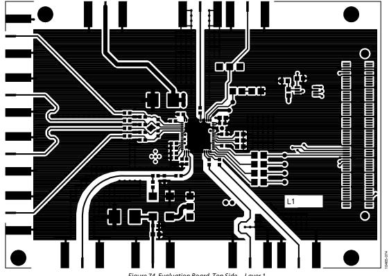
Figure 74. Evaluation Board, Top Side—Layer 1
