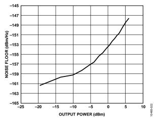
Figure 20. Noise Floor at 0 dB Attenuation vs. Output Power at Nominal Conditions
