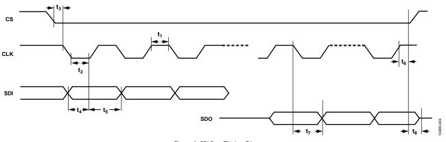
Figure 3. SPI Port Timing Diagram
