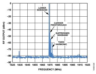
Figure 25. RF Output Spectral Plot over a 100 MHz Span
