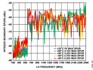
Figure 33. Integer Boundary Spur Performance vs. LO Frequency, Supply, and Temperature
