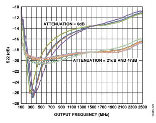
Figure 23. Output Return Loss at Different Attenuation Settings vs. Output Frequency, Supply, and Temperature
