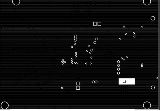
Figure 76. Evaluation Board, Ground—Layer 2
