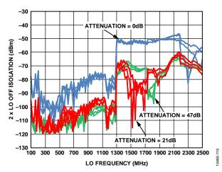
Figure 18.2 × LO Off Isolation vs. LO Frequency, Attenuation, Supply, and Temperature
