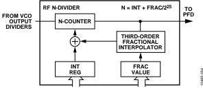
Figure 54. RF Fractional-N Divider
