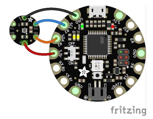
The SI1145 has a fixed I2C address (0x60), you can only connect one sensor per microcontroller!
