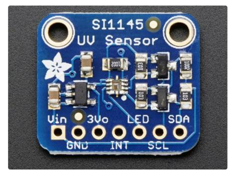
The SI1145 is an I2C sensor, so there are not a lot of pins to worry about.
