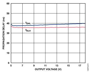
Figure 11. Typical Propagation Delay vs. Output Voltage,  $V_{DD1} = 5 V$
