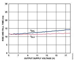
Figure 12. Typical Rise and Fall Time vs. Output Supply Voltage
