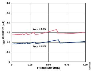
Figure 8. Typical IDD1 Current vs. Frequency
