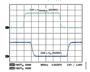
Figure 6. DISABLE to Output Waveform for 2 nF Load, 3.6  $\Omega$  Resistor with 12 V Output Supply,  $V_l = V_{DD1}$
