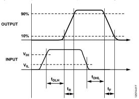
Figure 17. Propagation Delay Parameters
