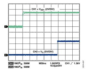
Figure 7. Typical  $V_{DD1}$  Delay to Output Waveform,  $V_1 = V_{DD1}$
