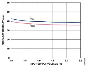
Figure 10. Typical Propagation Delay vs. Input Supply Voltage,  $V_{\text{DD2}} = 12 \text{ V}$
