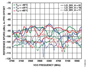
Figure 31. f<sub>PFD</sub> Spurs vs. VCO Frequency; 4× PFD Offset; Measured at LO Output
