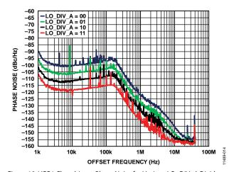
Figure 18. VCO1 Closed-Loop Phase Noise for Various LO\_DIV\_A Dividers vs. Offset Frequency;  $f_{VCO1} = 4.6 \text{ GHz}$
