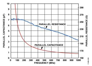
Figure 87. Mixer Output Impedance vs. Frequency
