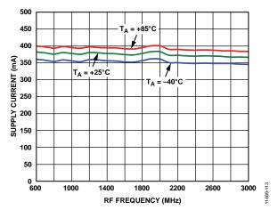
Figure 13. Supply Current vs. RF Frequency
