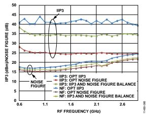
Figure 84. Example IIP3 and Noise Figure Optimization
