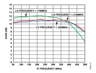
Figure 9. Gain vs. IF Frequency; RF Sweep with Fixed LO; IF and RF Roll-Off; Measured on 1 V p-p on Each Tone at DGA Output
