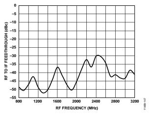
Figure 50. RF to IF Feedthrough at Mixer Output Without Filtering; Mixer Input Power = 0 dBm
