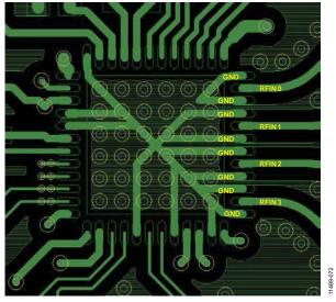
Figure 100. Recommended Layout for the RF Inputs
