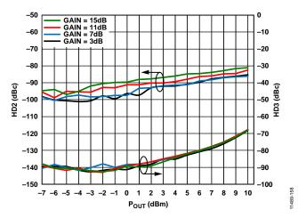
Figure 61. DGA HD2/HD3 vs. Output Power (Poυτ) and Gain Setting
