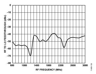
Figure 33. RF to LO Output Feedthrough, LO\_DRV\_LVL = 00
