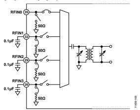
Figure 66. Terminating Unused RF Input Ports
