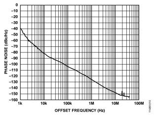
Figure 14. VCO2 Open-Loop VCO Phase Noise vs. Offset Frequency;  $f_{VCO2} = 3.4 \text{ GHz}$ ,  $LO\_DIV\_A = 00$ , VTUNE = 2V
