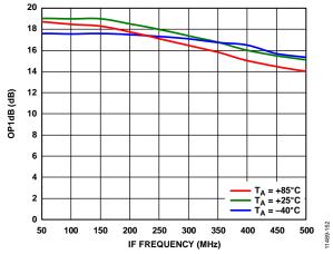
Figure 55. DGA OP1dB vs. Frequency and Temperature; Maximum Gain
