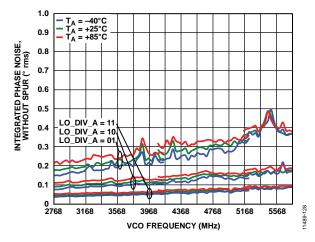
Figure 29. 10 kHz to 40 MHz Integrated Phase Noise vs. VCO Frequency; LO\_DIV\_A = 01, 10, and 11, Excluding Spurs, for Various LO Divider Ratios
