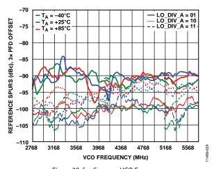
Figure 28.  $f_{PFD}$  Spurs vs. VCO Frequency;  $3 \times PFD$  Offset; Measured at LO Output
