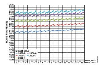
Figure 83. Noise Figure vs. MIXER\_RDAC, MIXER\_CDAC, and Various MIXER\_BIAS Values at RF Frequency = 2700 MHz
