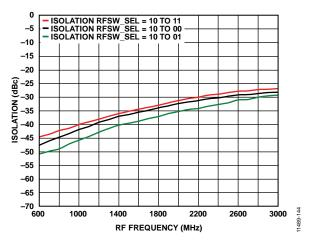
Figure 48. Mixer Input to Mixer Output Isolation vs. RF Frequency; RFSW\_SEL = 10 Driven
