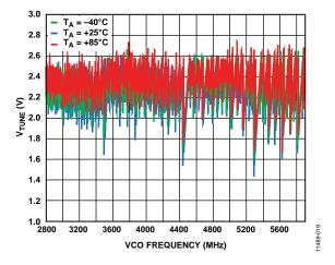
Figure 23. V<sub>TUNE</sub> vs. VCO Frequency
