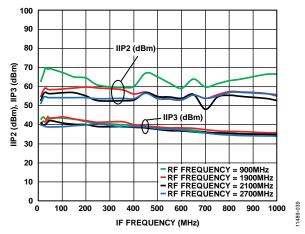
Figure 42. Mixer IIP2/IIP3 vs. IF Frequency;  $P_{IN} = -5$  dBm/Tone, 1 MHz Spacing, LO Sweep with Fixed RF, IF Roll-Off
