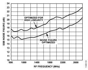
Figure 53. SSB Noise Figure vs. RF Frequency (see Table 16)
