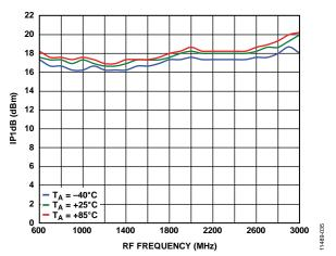
Figure 38. Mixer IP1dB vs. RF Frequency
