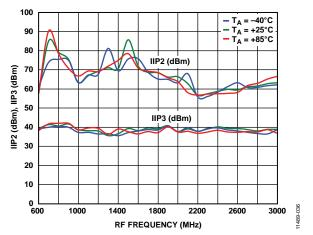
Figure 39. Mixer IIP2/IIP3 vs. RF Frequency;  $P_{IN} = -5$  dBm/Tone, 1 MHz Spacing
