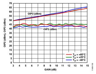
Figure 59. DGA OIP2/OIP3 vs. Gain Setting and Temperature
