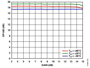
Figure 58. DGA OP1dB vs. Gain Setting and Temperature
