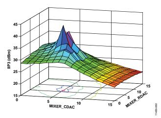
Figure 80. IIP3 vs. MIXER\_RDAC, MIXER\_CDAC; MIXER\_BIAS = 011 at RF Frequency = 2100 MHz
