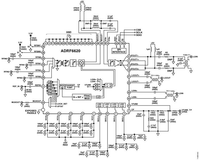
Figure 70. Basic Connection Diagram
