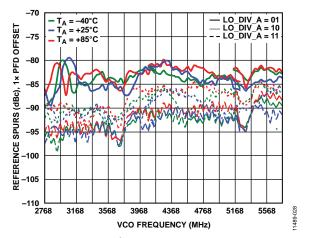
Figure 27. f<sub>PFD</sub> Spurs vs. VCO Frequency; 1× PFD Offset; Measured at LO Output
