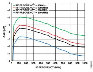
Figure 40. Mixer Gain vs. IF Frequency; LO Sweep with Fixed RF, IF Roll-Off
