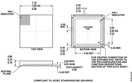
Figure 102. 48-Lead Lead Frame Chip Scale Package [LFCSP\_WQ]
