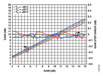
Figure 57. DGA Gain and Gain Step Error vs. Gain Setting and Temperature
