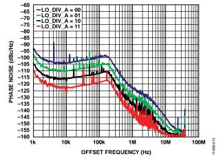
Figure 17. VCO2 Closed-Loop Phase Noise for Various LO\_DIV\_A Dividers vs. Offset Frequency;  $f_{VCO2} = 3.4 \text{ GHz}$
