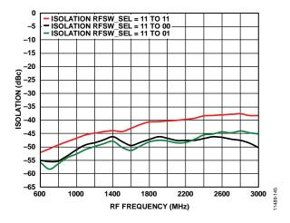
Figure 47. Mixer Input to Mixer Output Isolation vs. RF Frequency; RFSW\_SEL = 11 Driven
