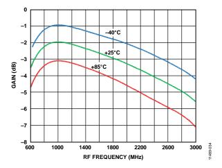
Figure 37. Mixer Gain vs. RF Frequency
