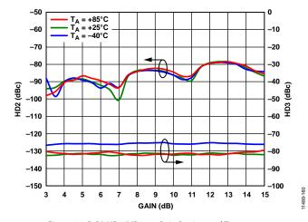
Figure 63. DGA HD2/HD3 vs. Gain Setting and Temperature
