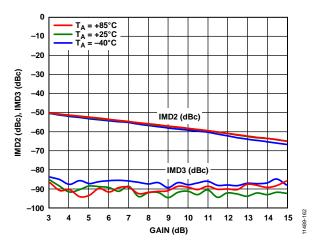
Figure 65. DGA IMD2/IMD3 vs. Gain Setting
