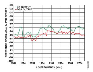
Figure 36.  $f_{PFD}$  Spurs, LO\_DIV\_A = 01, 1× PFD Offset; Measured on LO Output and DGA Output
