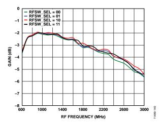
Figure 43. Mixer Gain vs. RF Frequency; RFSW\_SEL = 00, 01, 10, and 11
