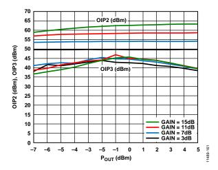
Figure 64. DGA OIP2/OIP3 vs. Output Power (Pout) and Gain Setting
