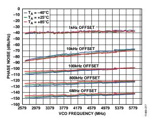
Figure 21. Open-Loop Phase Noise vs. VCO Frequency;  $LO\_DIV\_A = 00$
