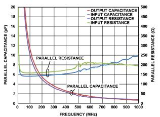
Figure 88. IF DGA Input/Output Impedance vs. Frequency
