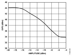
Figure 89. OIP3 vs.  $(f_{RF} + f_{LO})$  Amplitude
