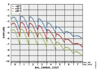
Figure 73. Gain vs. BAL\_CIN and BAL\_COUT at RF = 1900 MHz
