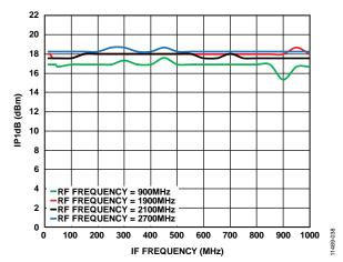
Figure 41. Mixer IP1dB vs. IF Frequency; LO Sweep with Fixed RF, IF Roll-Off
