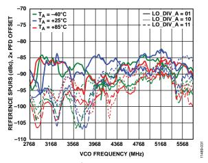
Figure 30. f<sub>PFD</sub> Spurs vs. VCO Frequency; 2× PFD Offset; Measured at LO Output
