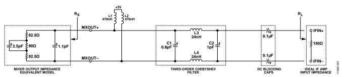
Figure 91. Low-Pass Interstage Filter Design
