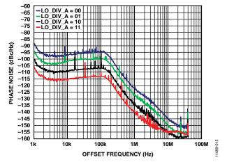
Figure 19. VCO0 Closed-Loop Phase Noise for Various LO\_DIV\_A Dividers vs. Offset Frequency;  $f_{VCO0} = 5.532$  GHz
