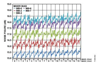
Figure 78. Noise Figure vs. MIXER\_RDAC, MIXER\_CDAC, and Various MIXER\_BIAS Values at RF Frequency = 900 MHz
