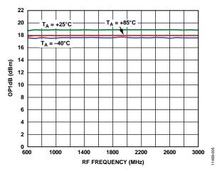
Figure 5. OP1dB vs. RF Frequency
