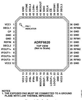
Figure 3. Pin Configuration
