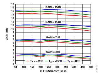
Figure 54. DGA Gain vs. IF Frequency and Temperature
