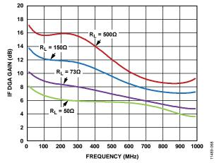
Figure 95. IF DGA Gain vs. Frequency for Different Loads
