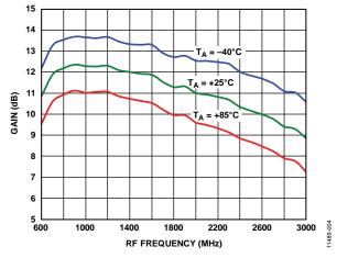
Figure 4. Gain vs. RF Frequency; IF Frequency = 200 MHz
