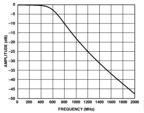
Figure 98. Simulated Antialiasing Filter Design
