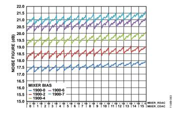
Figure 79. Noise Figure vs. MIXER\_RDAC, MIXER\_CDAC, and Various MIXER\_BIAS Values at RF Frequency = 1900 MHz
