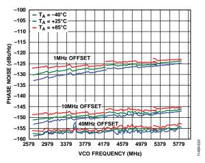
Figure 24. Open-Loop Phase Noise vs. VCO Frequency;  $LO\_DIV\_A = 00$
