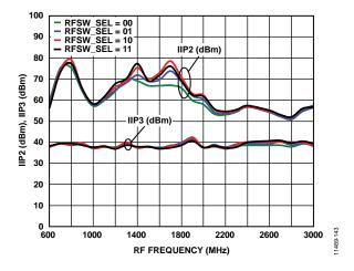
Figure 46. Mixer IIP2/IIP3 vs. RF Frequency; RFSW\_SEL = 00, 01, 10, and 11
