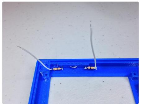
Then solder each of them to the outer two pins of the pushbuttons. The 4cm wire on the left, 5cm on the right.
