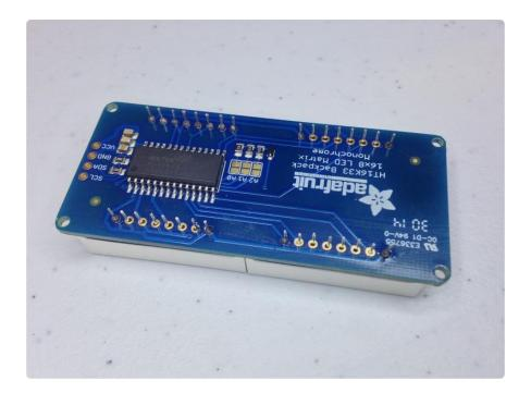
Let's start with the soldering the LED matrices to the Backpack. After all 32 pins have been soldered, carefully trim the pins with a flush cutter.
