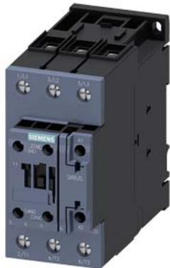
power contactor, AC-3 40 A, 18.5 kW / 400 V 1 NO + 1 NC, 110 V AC 50 Hz / 120 V, 60 Hz, 3-pole, Size S2, screw terminal
