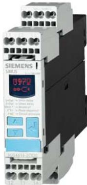
Digital monitoring relay 3-phase supply voltage Phase sequence can be activated Phase failure 3 x 160 to 690 V 50 to 60 Hz AC Undervoltage and overvoltage 160-690 V Hysteresis 1-20 V 0-20 s each for Umin and Umax 1 CO for Umin 1 CO for Umax spring-type connection system
