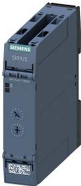
Timing relay, electronic OFF delay without control signal or smooth passing make contact non-volatile 7 time ranges 0.05...600 s 24 V AC/DC, 2 change-over contacts with LED, Screw terminal
