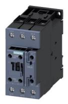
Power contactor, AC-3 65 A, 30 kW / 400 V 1 NO + 1 NC, AC / DC 20-33 V, with varistor 3-pole, size S2 screw terminals
