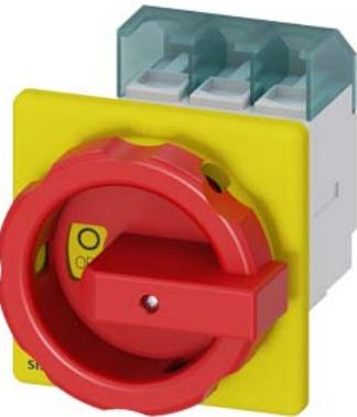
SENTRON, Switch disconnector 3LD, emergency switching-off switch, 3-pole,  $I_{u}$ : 63 A, operating power / at AC-23 A 400 V: 22 kW, front-mounted, rotary operating mechanism, Red / yellow, central mounting 22.5 mm of the handle
