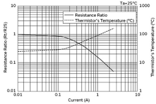
Current-R ratio( $R_t/R_{25}$ ), Current-Temperature Characteristics
