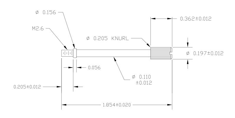
FOR USE IN SERIES\*\* #'S: 952, 970, 971\*, 972 \*FOR 971, CAN ONLY BE USED TO REPLACE (1) SCREW DUE TO INTERFERENCE \*\* PLEASE ENSURE FIT AND FUNCTION ARE SUITABLE FOR YOUR APPLICATION
