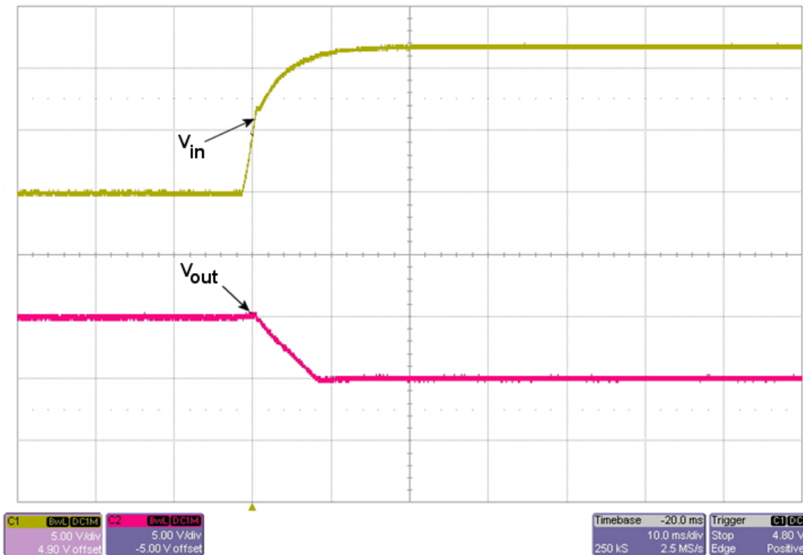
Figure 6. Power Up, V_{OUT} Relative to V_{IN}
