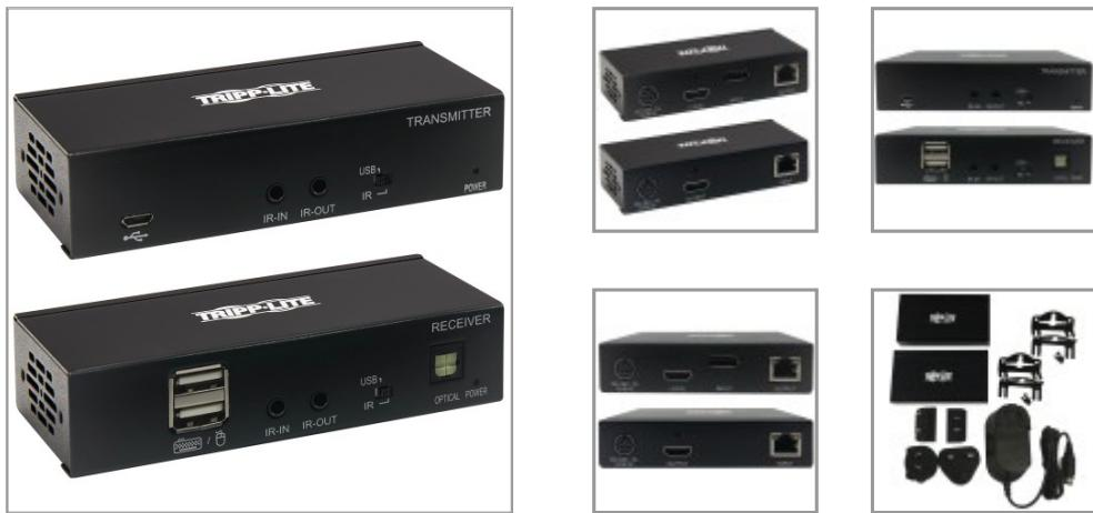
Transmitter/receiver kit extends a 4K signal via Cat6 cable from a DisplayPort source to an HDMI display up to 230 ft. away.
