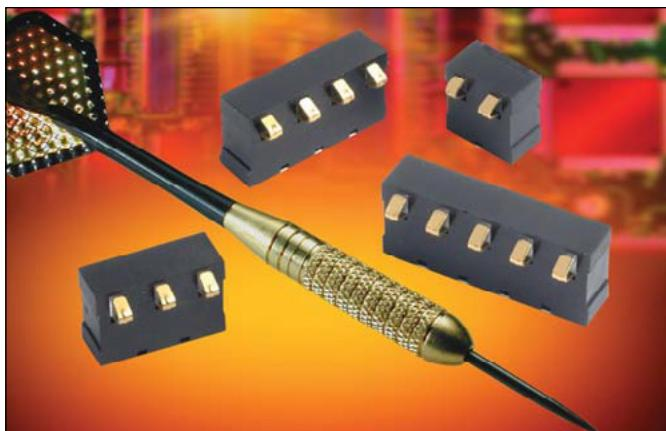
A further addition to the battery connector range offered by KYOCERA AVX is a 90 degree version. On a 3mm pitch, offered in 2 to 6 contact positions and rated as with all of the battery range at 3 amps. The connector's design is small and compact to minimize its profile yet stable while having a contact point 4.61mm above the PCB.
