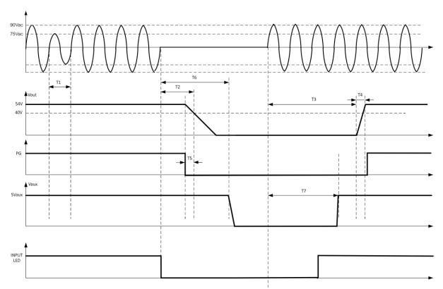
T1 – ride through time – 0.5 to 1 cycles [ 10 - 20ms] V<sub>OUT</sub> remains within regulation – load dependent
