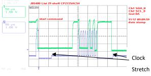
Example waveforms showing clock stretching.
