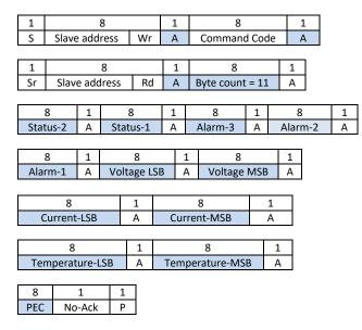
Status\_unit(0xD1): This command returns the STATUS-2 and STATUS-1 register values using the standard 'read' format. Status-2
