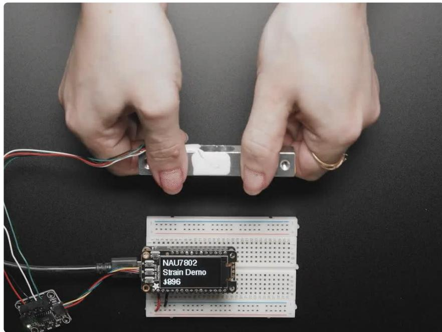
If you are feeling the stress and strain of ~~modern life~~ a Wheatstone bridge and you want to quantify it, this handy breakout will do the job, no sweat! The Adafruit NAU7802 contains a super-high-resolution 24-Bit differential ADC with extra gain and calibration circuitry that makes it perfect for measuring strain gauges / load cells or other sensors that have four wires that are connected in a [Wheatstone bridge arrangement](https://adafru.it/-kd) (<https://adafru.it/-kd>).
