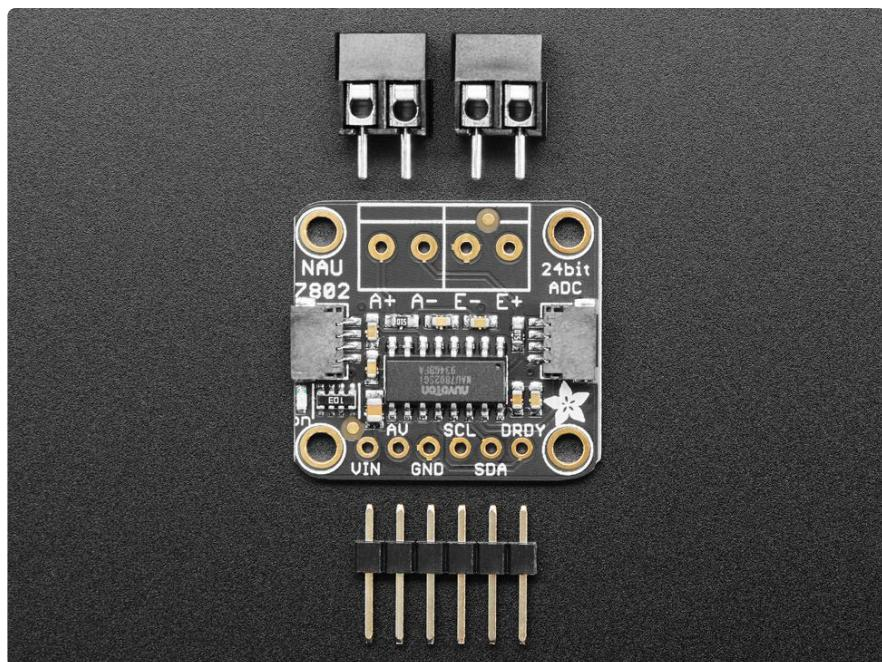
Each breakout comes with a NAU7802 ADC chip, plus some support circuitry, and 4 terminal blocks that can be used to connect a 4-wire sensor.
