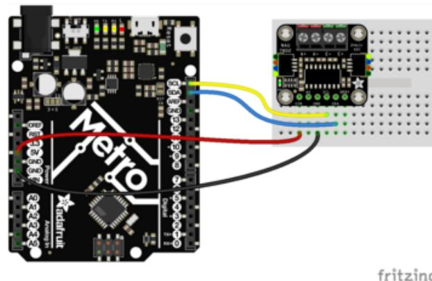
Board 5V to ADC VIN (red wire)
