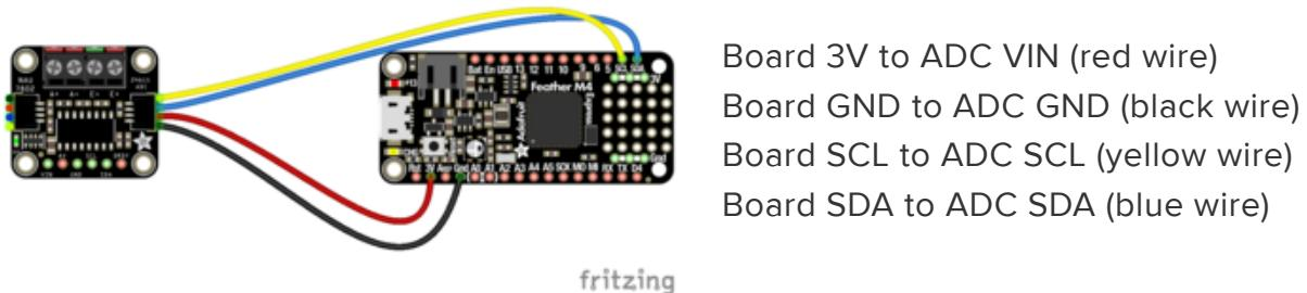
You can also use the standard 0.100" pitch headers to wire it up on a breadboard:
