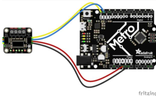
Board 5V to ADC VIN (red wire)
