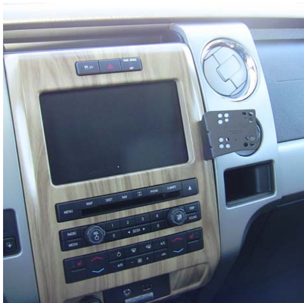
InDash installed showing location
