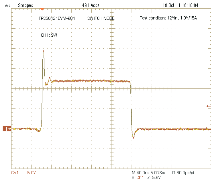
Figure 9-5. Switch Node Waveform Measured at Pins Using Tip and Barrel Measurement Technique (VIN = 12 V, VOUT = 1.0 V, IOUT = 15 A)
