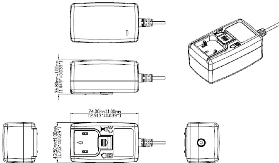
LED INDICATOR: Green Power ON indicator LED standard. May be ordered without LED as an option, for cost reduction.
