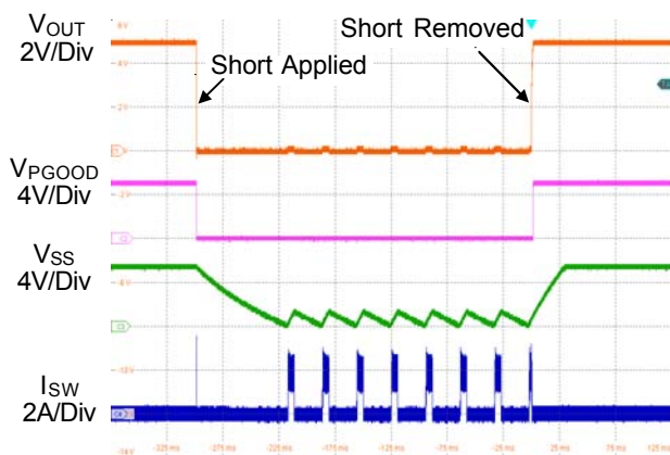
Figure 3. Short Circuit Protection and Recovery
